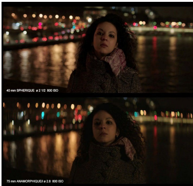
Figure 7 – the same composition shot, only with a spherical vs anamorphic lens. (9)
